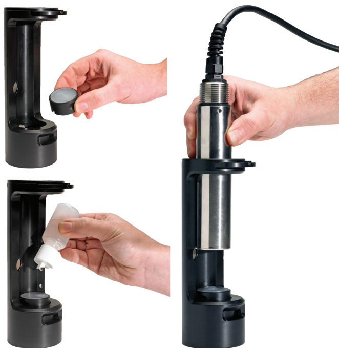
Figure 6 ATS430 easy calibration procedure
